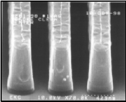
Figure 2a: 0.23-micron Metal Line (Oxide/Ti/TiN/AlCu/TiN) - Before Clean
