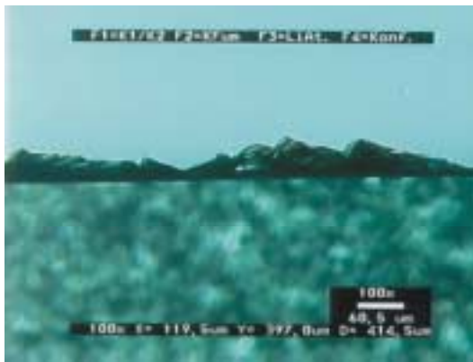
Fig. 1: Micro-cracks along dicing line after sawing a 30 \mu\text{m} thin wafer.
